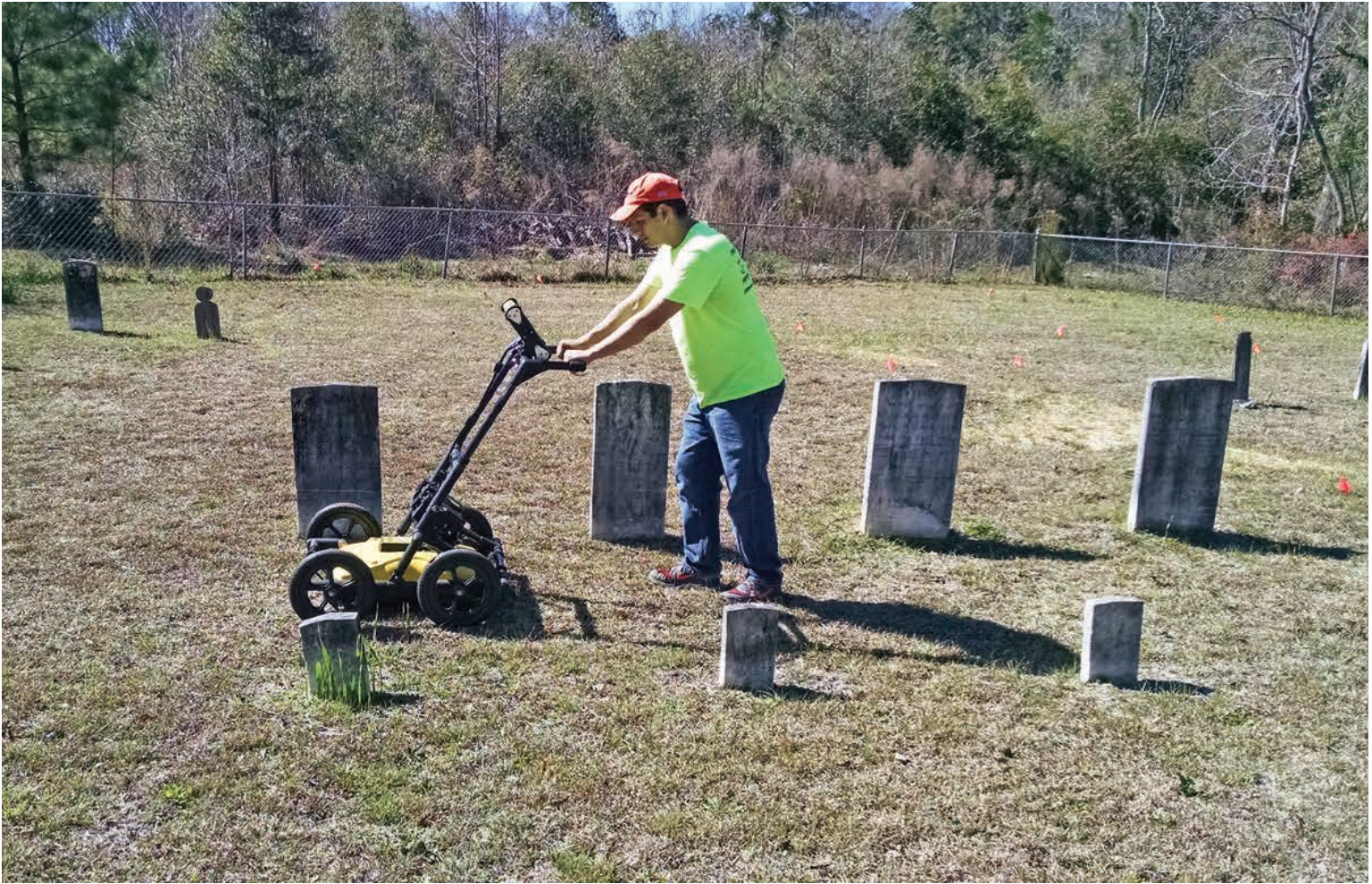
ABOVE: NOT MOWING THE LAWN – A MEMBER OF THE BIGMAN GEOPHYSICAL TEAM USES GPR TO VISUALIZE THE “KNOWN” PARTS OF THE CEMETERY TO HELP HIM LATER CHART THE UNKNOWN PARTS. RIGHT: A LOOK AT WHAT A GPR OPERATOR SEES ON THE SCREEN. (PHOTOS COURTESY BIGMAN GEOPHYSICAL)
